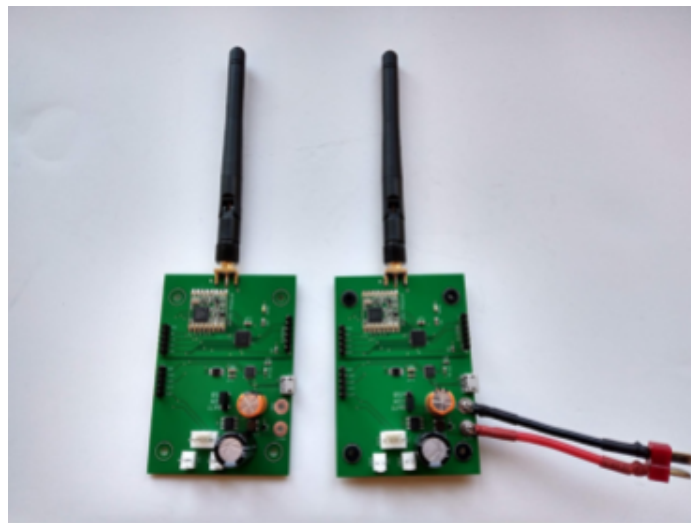
Figure 3: Assembled Receiver (left) and Transmitter (right) boards
